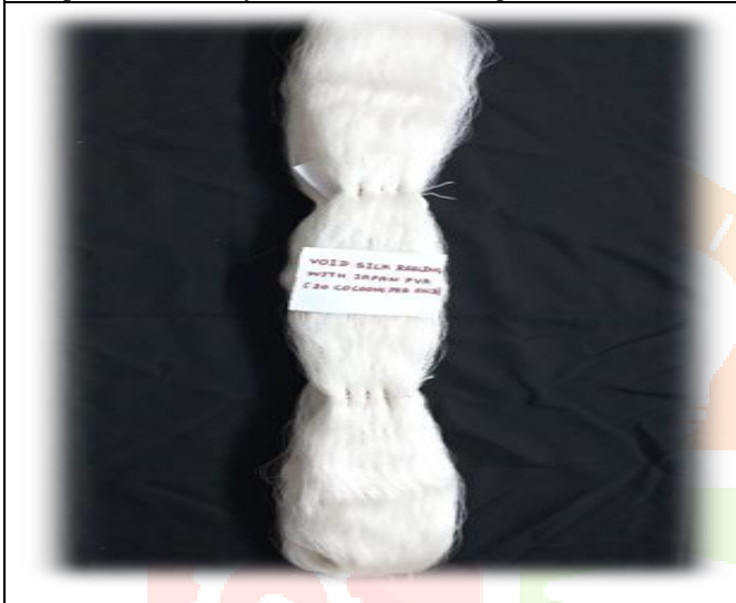
Fig. 3 a. The bulky void raw silk yarn produced with 20 cocoons and Indian PVA yarn.
