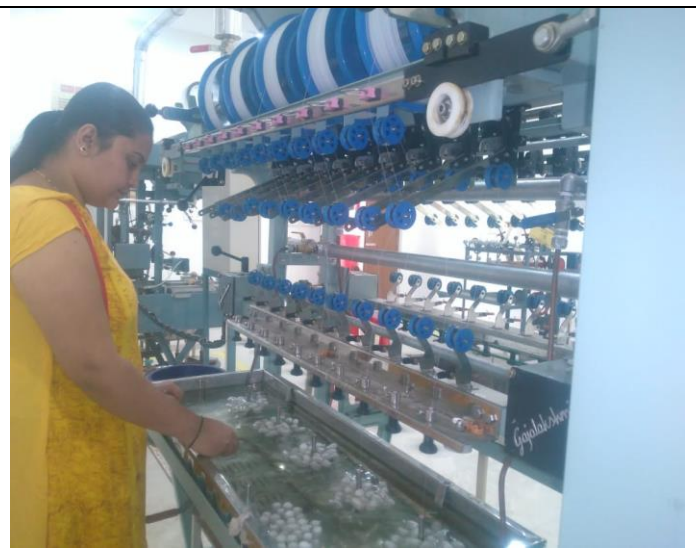
Fig. 2. Modified multiend reeling machine for the production of bulky void raw silk yarn along with PVA yarn.
