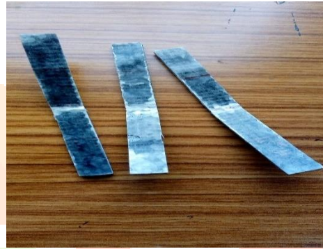
Fig :11 Flexural Test Breaking specimens
