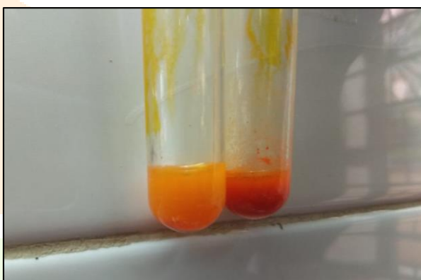
Fig -9: Confirmatory test for caffeine Left tube: 'Control' tube (yellow colour) Right tube: 'Test' tube (orangish-red colour)
