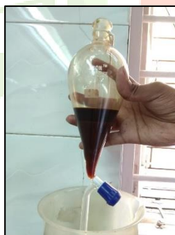
Fig -5: Upon cooling, it was transferred into a separating funnel. 10 ml DCM was slowly poured into the funnel and the 2 layers were mixed by gently stirring them for about 5 minutes.
