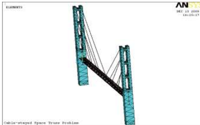
Fig.1 Cable-stayed space truss model built in ANSYS
