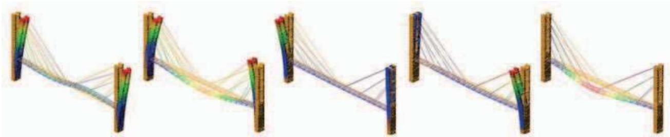
Fig.2 Mode shapes from 1st order to 5th order in ADAMS.
