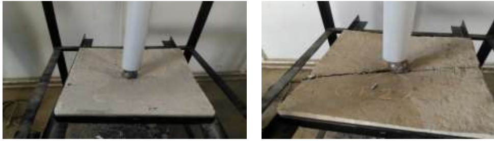
Fig. Initial and Final cracking of slab panel
