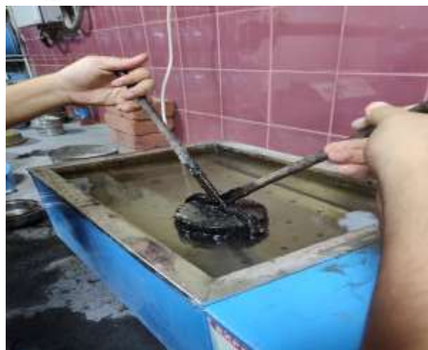
Figure 4.4: Water Bath Machine (At 60^{\circ}\text{C} \pm 1\% of set point for 30 min.)
