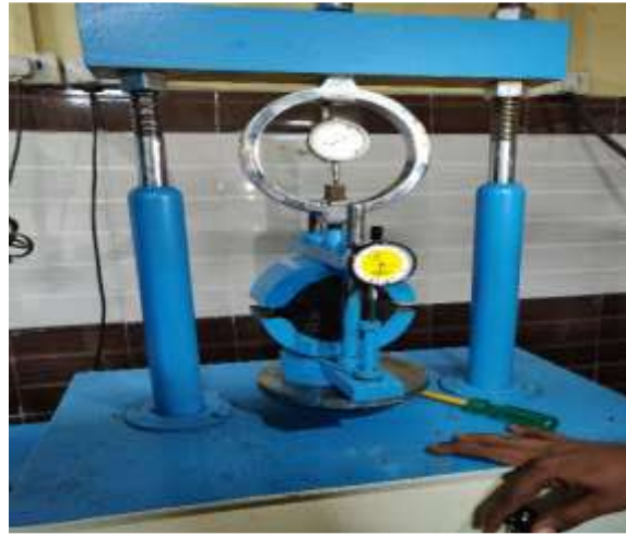
Figure 4.5: Marshall Stability Testing.
