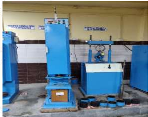
Figure 4.2: Asphalt Concrete Compaction
