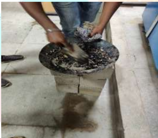
Figure 4.1: Mixing of Asphalt Concrete With PKS
