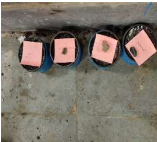
Figure 4.3: Asphalt Concrete mould after Compaction. (Kept in mould for 24 hour)
