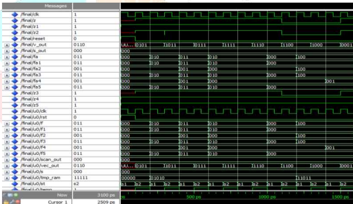
Fig 13: Simulation Output for Stuck-At Fault model for Bit Swapping LFSR
