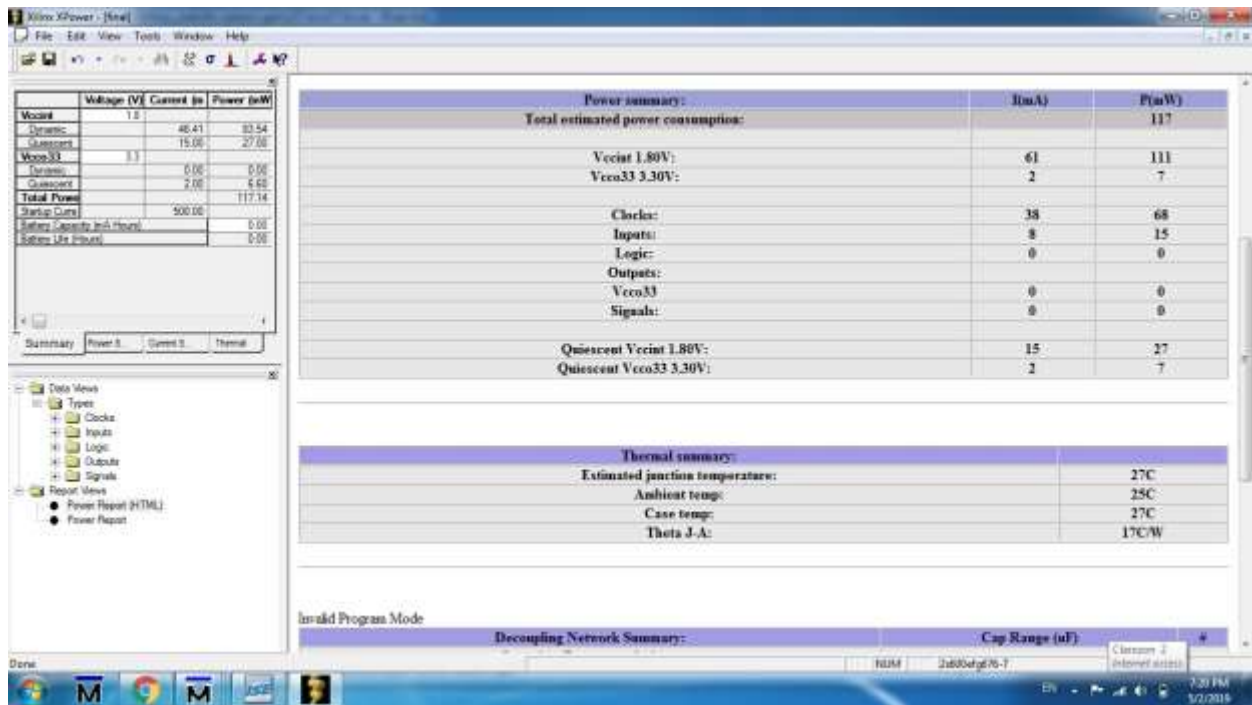
Fig 16: Power Results for S27 Circuit with Bit-Swapping LFSR
