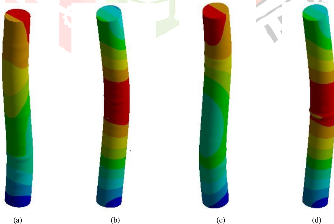
Fig -1: Total deformation of outer prismatic inner non-prismatic CTSRC columns: (a) L shape, TR=1.2, (b) L shape, TR=0.8, (c) V shape, TR=1.2, (d) V shape, TR=0.8
