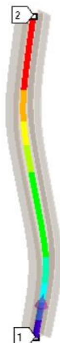
Fig -3: Total Deformation along the path of outer prismatic inner non-prismatic CTSRC column (L shape, TR=1.2)
