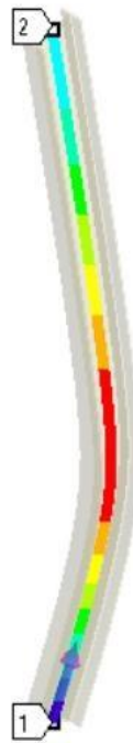
Fig -4: Total Deformation along the path of outer non-prismatic inner prismatic CTSRC column (V shape, TR=1.2)
