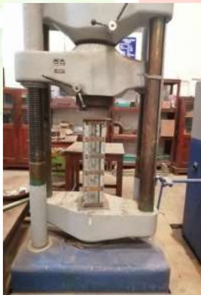
Fig -4: Test Setup for Compression Test
