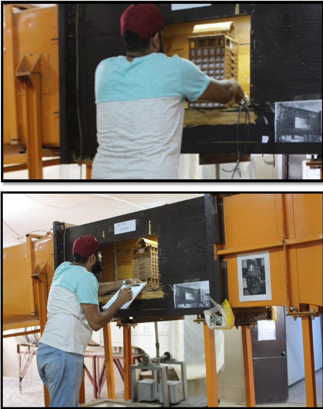
Figure (8) Photographs Showing the Laboratory Horizontal Wind Tunnel Baghdad University Tower Model.
