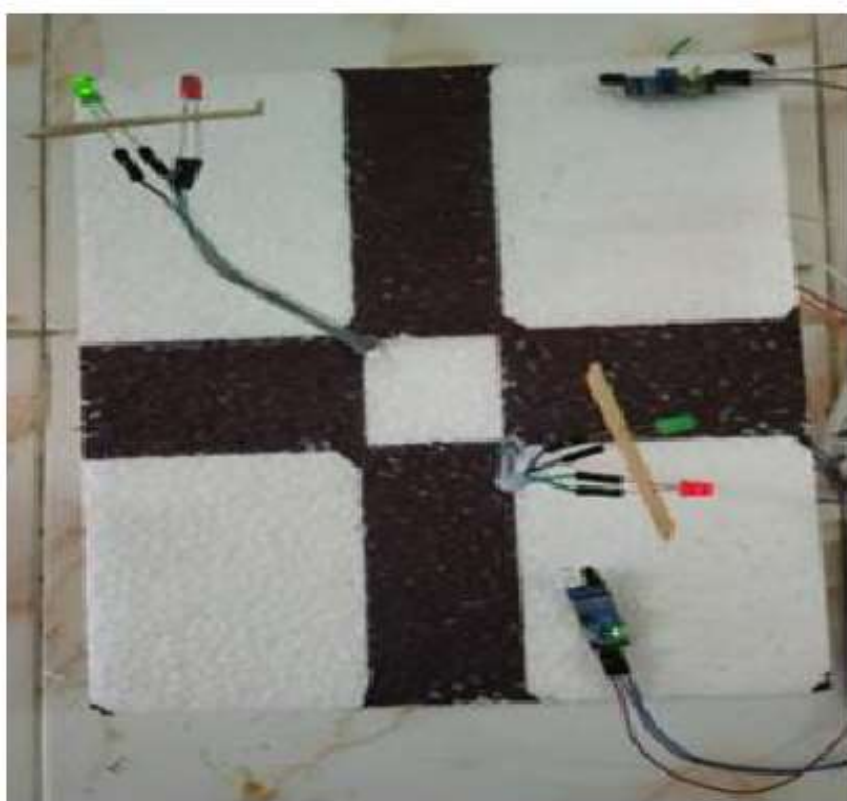
Figure 7: Traffic system circuit
