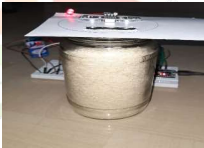
Fig: Dustbin is empty red light is off (left), Dustbin status-full red light is on (right)
