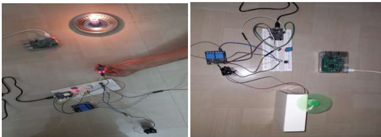
Figure 11: flame detection (left), temperature and humidity detection (right)
