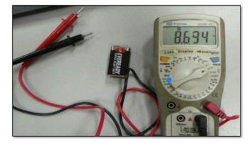
Fig. 3: Battery voltage measurement using multimeter
