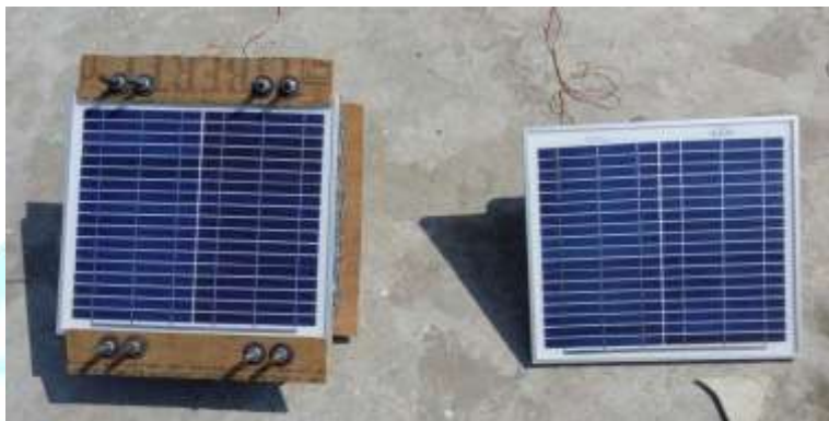
Fig: 2.5 Experimental setup(PV panel with & without cooling)
