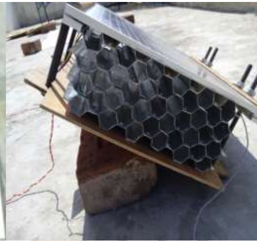
Fig: 2.2 Panel with honeycomb fins
