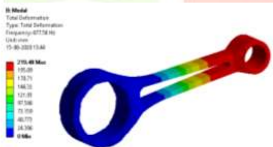
Fig 6.1: First mode of Connecting rod
