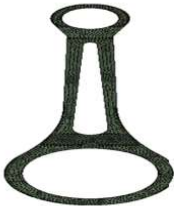
Fig 4.1: Connecting Rod with Cut out.
