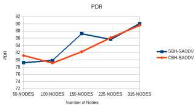
Figure-12 Packet Delivery Ratio comparison for single and Cooperative blackhole attacks with respect to number of node variation using Secure-AODV.
