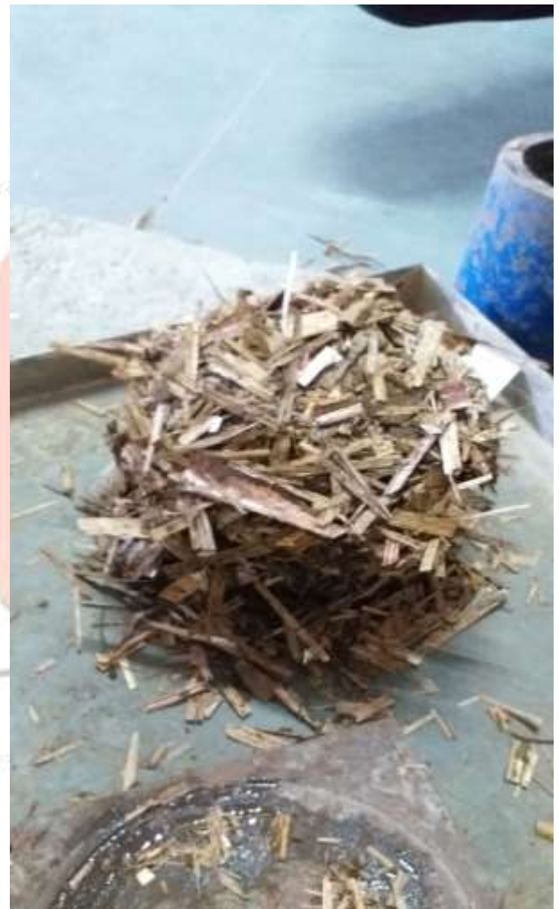
Fig no. 9 briquette fall in pieces
