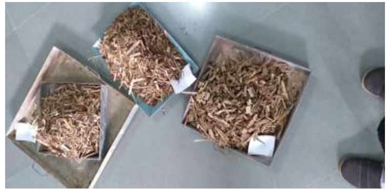
Fig no. 8 size reduction up to 5-6 cm
