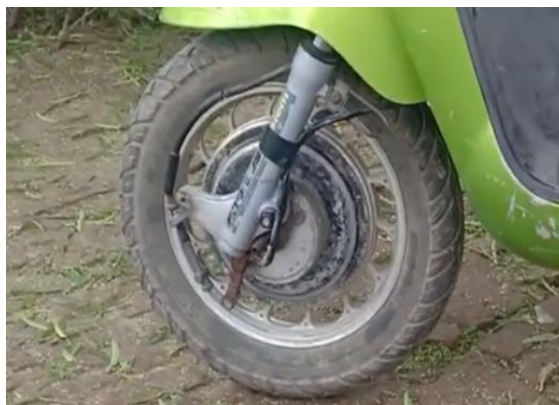
Fig. 4: Real time photo BLDC hub motor on front Wheel of scooty.
