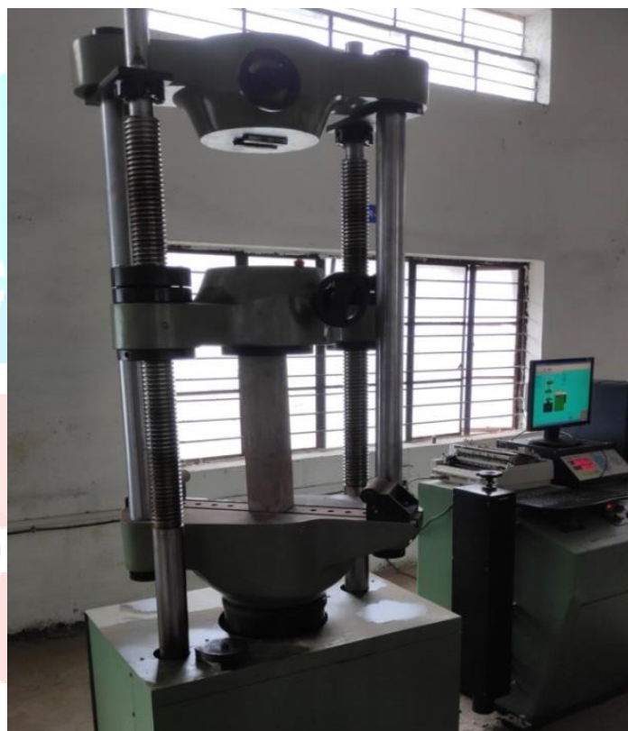
Figure 2. Test Setup For Column On UTM Machine
