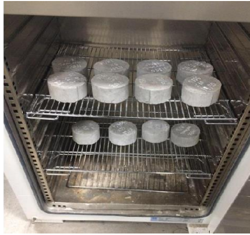
Figure 4.6 - Samples kept in Oven
