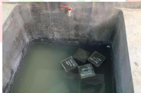
Figure 4.5 – Samples cured in a water tank
