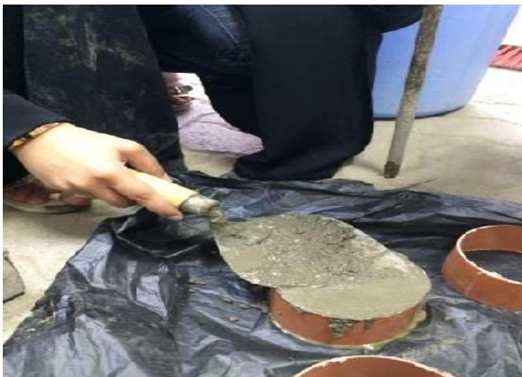
Figure 4.3 – Levelling Cylindrical Samples with trowel
