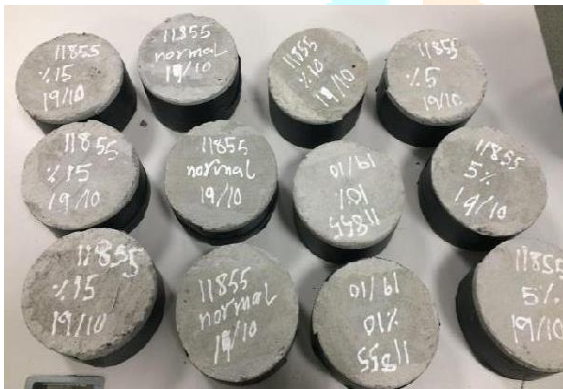
Figure 4.7 – Peripheral surface covered with tape
