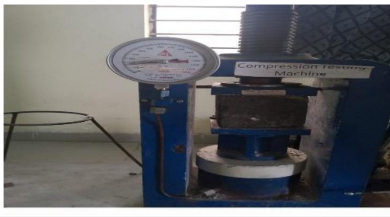
FIGURE NO: 3 Compressive strength test is performed by comprehensive strength test machine
