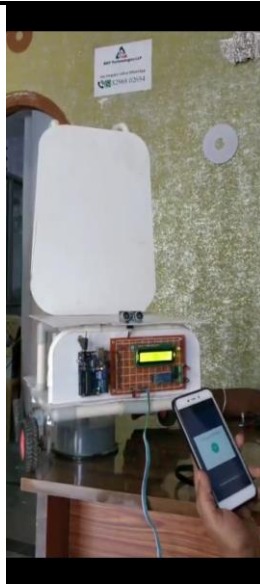
Fig No 4. Giving the voice commands to move the wheelchair in different directions.
