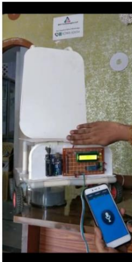
Fig No 5. Using the ultrasonic sensor to stop the wheelchair if any obstacles are present.
