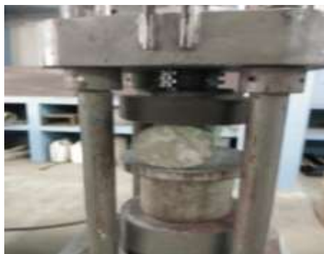
FIGURE 4 Tensile Strength Test Setup
