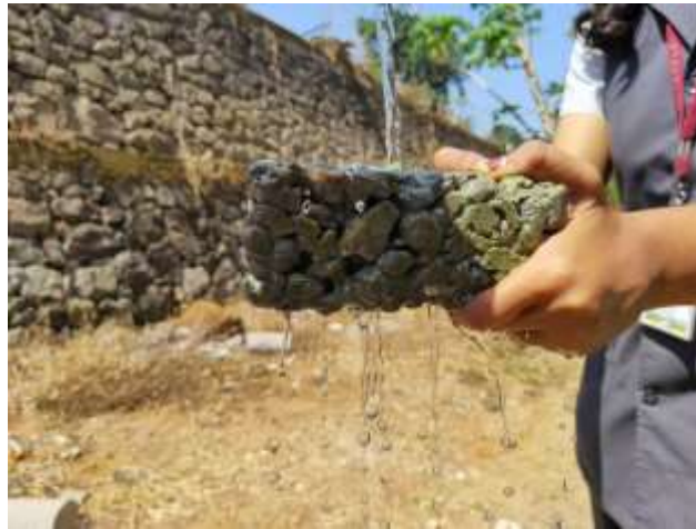
Fig.2 Pervious concrete block
