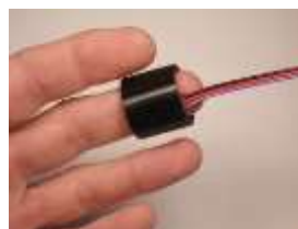
Fig. 1 the Pulse sensor is held to the finger.
