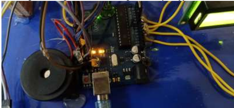
Fig 15: Buzzer which activates on first warning
