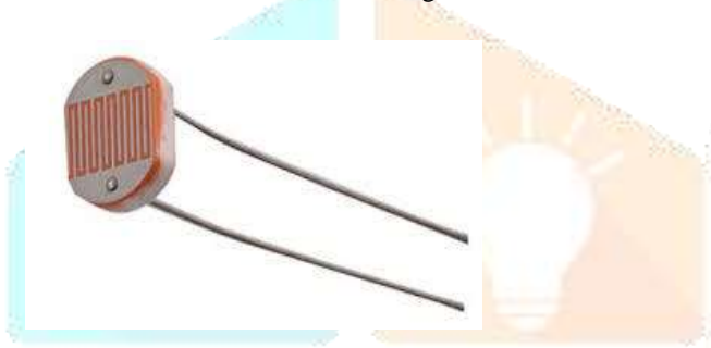
Figure 3: Light Dependent Resistor (LDR) sensor.
