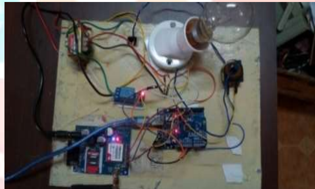
Figure 4: Prepaid energy meter by using GSM Technology without load.
