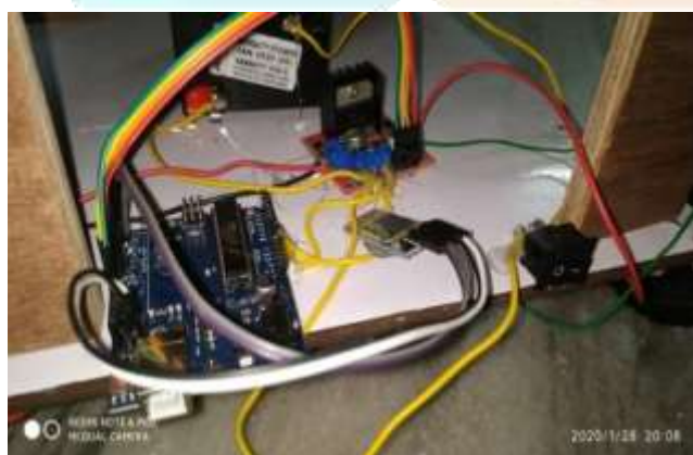
Fig 7: Interfacing of Arduino uno, Bluetooth, L298 and battery
