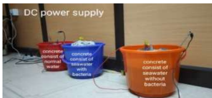
Fig 4.4: Laboratory setup of Impressed voltage test
