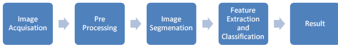
Figure 1 Steps in surface defect detection
