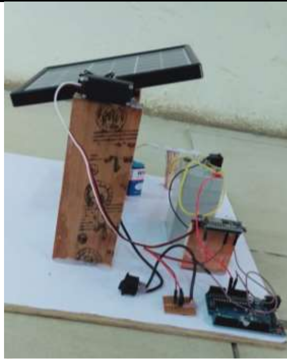
Fig: Solar panel is rotating according to the position of the sun
