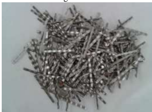
Fig. 1 Flat crimped macro steel fibres Table 1 Specification of flat crimped macro fibres
