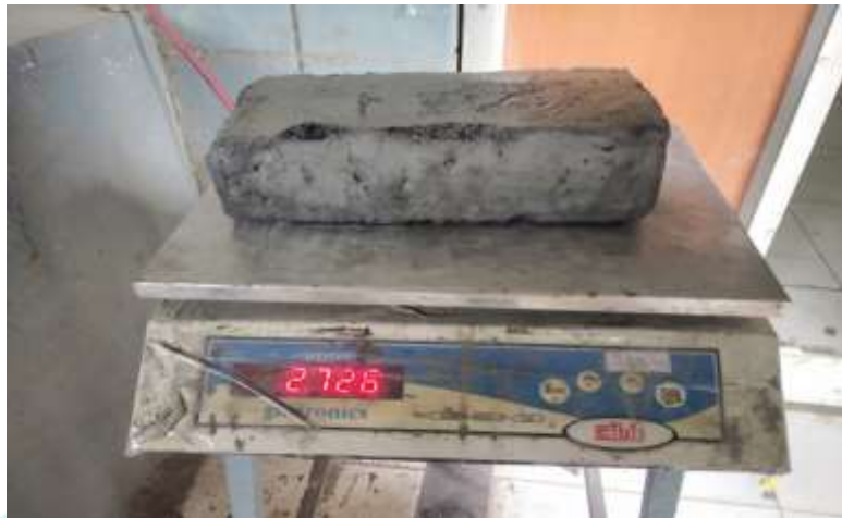
Fig 8 Water absorption test
