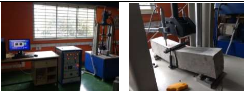
Figure 2 Fatigue testing machine and Failure of beam after fatigue test
