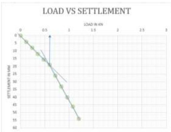
Figure 2 Load settlement graph for model footing Resting on soft clay without cement grout
