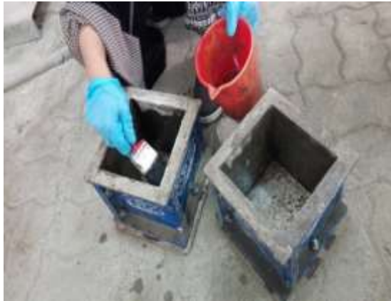
Figure 3.8 cleaning & greasing the cube moulds
