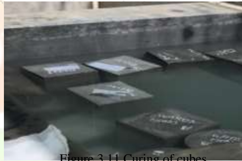
Figure 3.11 Curing of cubes
