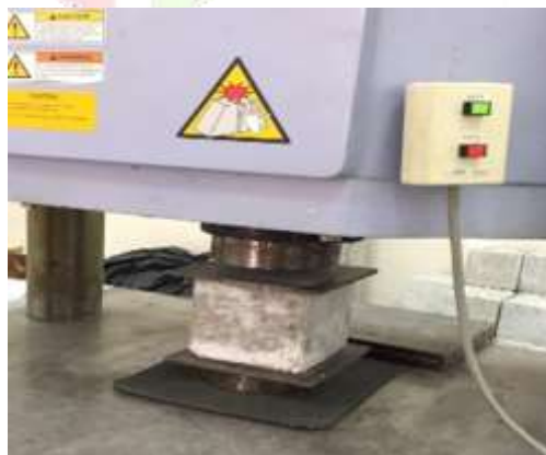
Figure 3.12 Compression Test in Progress
