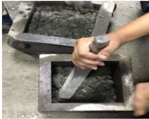
Figure 3.9 Compaction of concrete in cube sample
