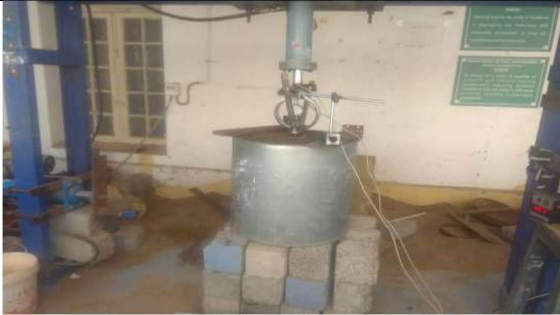
Experimental setup for vertical loading
