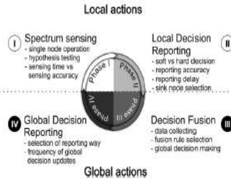
Fig. 2. Cooperative spectrum sensing procedure. However, several investigations pointed out that sensing carried out locally by single devices is not accurate enough for the safe coexistence of primary and secondary users. Thus, it is generally agreed that one of the ways to increase the reliability of spectrum sensing is to apply cooperation between nodes. In cooperative spectrum sensing every node in a cognitive network senses the spectrum, and reports local sensing results, which are then used for acquiring a global decision characterized by the global probability of detection (see Fig. 2). In the following subsections each of these phases will be discussed in detail.
