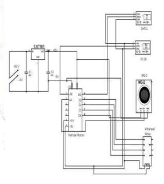
The figure shows hardware style establish with a 220V to 12V DC adapter that is linked to AN IC LM7805 that could be a 12V to 5V regulator. The fiberboard and therefore the device MQ2 is powerdriven with the 5V. The alternative sensors are power-driven by the 3v pin that's current within the fiberboard.
