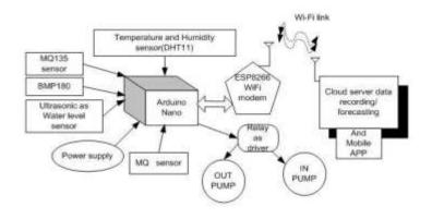
The block diagram consists of Arduino, Wifi Module, MQ Sensor, Temperature and Humidity Sensor, Water level Sensor, Soil Moisture Sensor,
