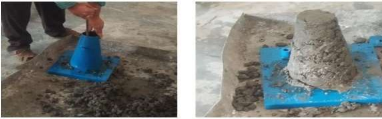
Figure6 (a) Tampering of materials in the slump cone Figure6 (b) slump of concrete mix on the tray.
