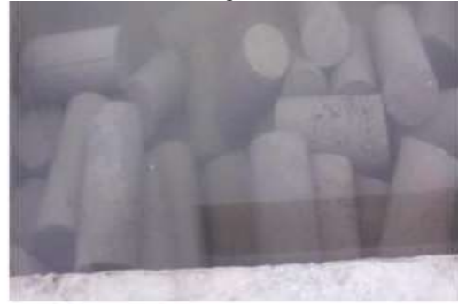
Figure 7.2 (b): specimens in the curing tank
