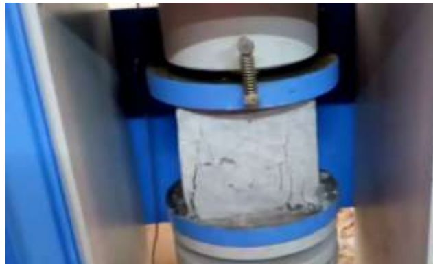
Figure 7.3: Compressive strength test setup
