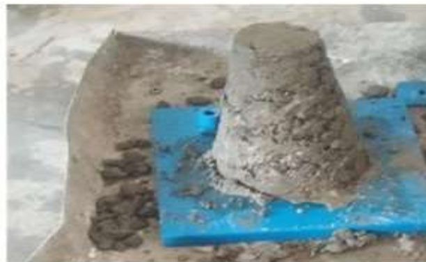
Figure6 (a) Tampering of materials in the slump cone Figure6 (b) slump of concrete mix on the tray.
