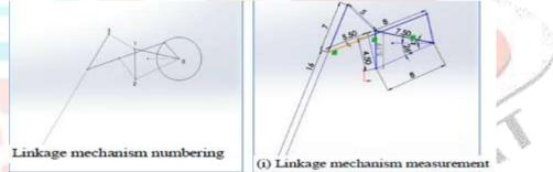
Diagram of Klann linkage mechanism showing numbering system and optimized linkage lengths to be used later in this analysis. In this paper hinge 0 may be called "the crank" and hinge 3 may be called "the foot." Hinges 0, 1 and 2 have fixed positions relative to each other for the entire locomotive cycle; the convention in this analysis will be fix hinge 0 at the origin and hinge 1 and 2.
