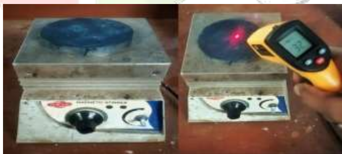
Fig. 2.3 Measure the temperature of coating component
