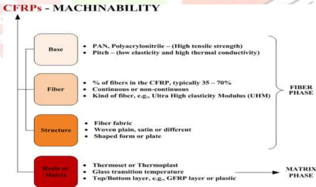
Fig 1: Material properties of CFRPs governing the machinability of CFRPs [32]
