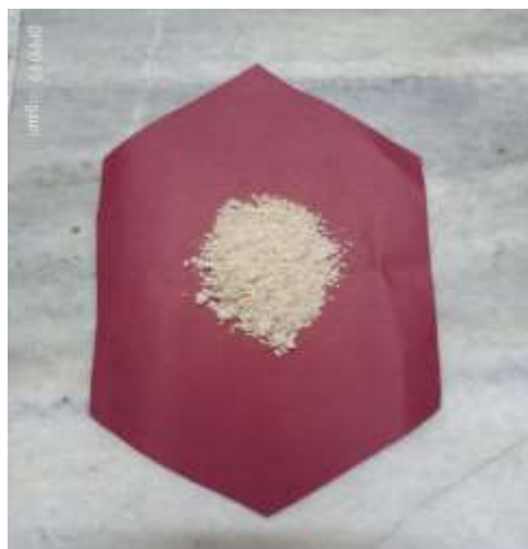
Fig 3: biopolymer from maranta arundinacea (arrowroot)
