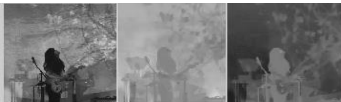
Figure 4.3: Separation of YCbCr Converted Image into Three Components (Luminance, Chrominance and Chromatic)
