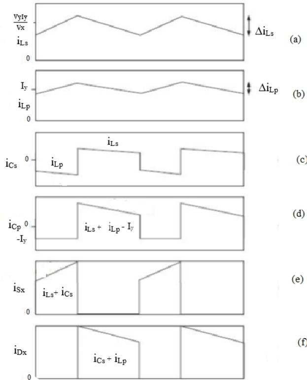
Fig.4 a. Current through Inductor Ls (iLs), b. Current through Inductor Lp (iLp), c. Current through Capacitor Cs (iCs), d. Current through Capacitor Cp (iCp), e. Current through switch Sx (iSx), f. Current through diode Dx (iDx).
