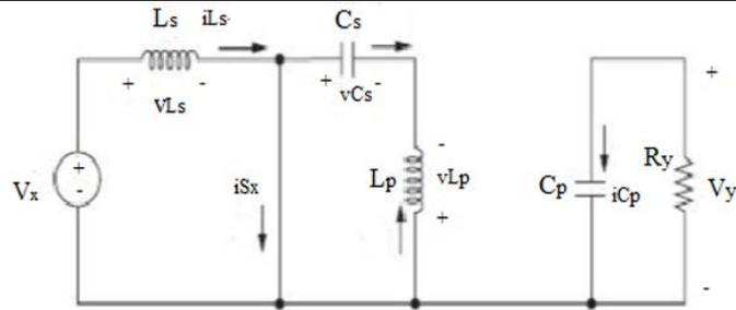
Fig.2 SEPIC Circuit with the switch closed
