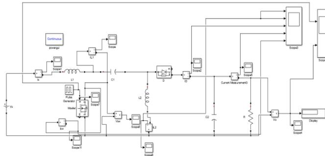
Fig.6 Simulation of open loop SEPIC converter
