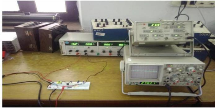
Fig.10 Hardware setup of SEPIC converter for closed loop system
