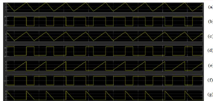
Fig.8 a. Current through Inductor Ls ( $iL_s$ ), b. Voltage across Inductor Ls ( $vL_s$ ), c. Current through Inductor Lp ( $iL_p$ ), d. Voltage across Inductor Lp ( $vL_p$ ), e. Current through switch Sx ( $iS_x$ ), f. Voltage across switch Sx  $vS_x$ , g. Current through diode Dx ( $iD_x$ ).
