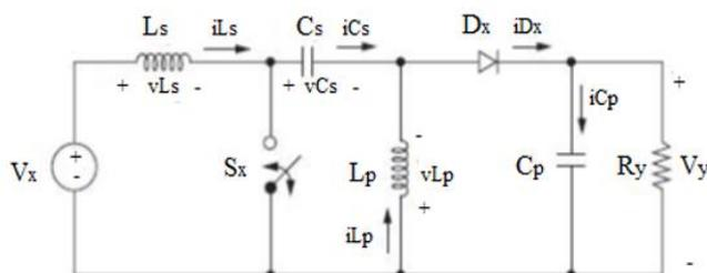
Fig.1 Proposed SEPIC converter schematic diagram.
