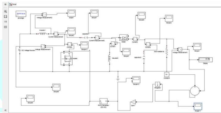
Fig.7 Simulation of closed loop SEPIC converter
