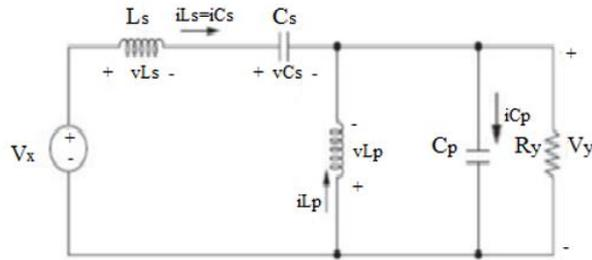
Fig.3 SEPIC Circuit with the switch open
