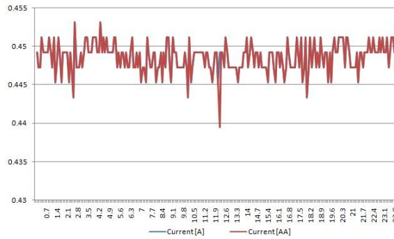
Graph 18: Actual Current to Apparent Current
