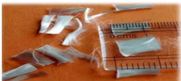
Figure: 4 Polypropylene fibres showing 12 mm average size
