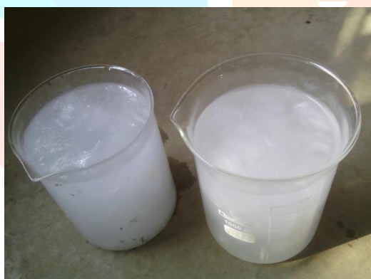
Figure: 5 Dispersion of PP fibres in NaOH solution
