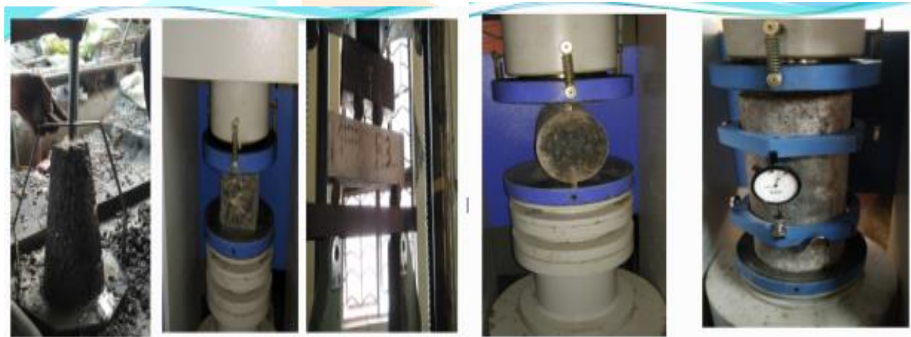
Fig 3.2 slump test, compression test, flexural test, split tensile test, modulus of elasticity
